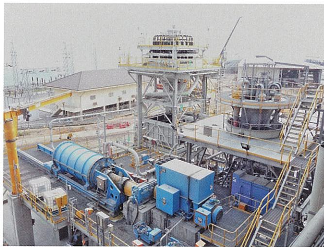
Jameson Cell in a cleaner scalping duty at Phu Kham, Laos, producing final grade copper concentrate prior to conventional cleaning circuit (flowsheet presented in May at Austmine 2011, Brisbane)
